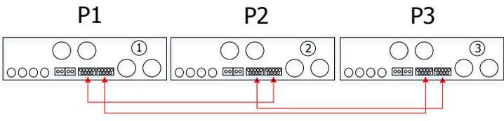
**WARNING:** Do not connect the current sharing cable between the inverters which are in different phases. Otherwise, it may damage the inverters.
