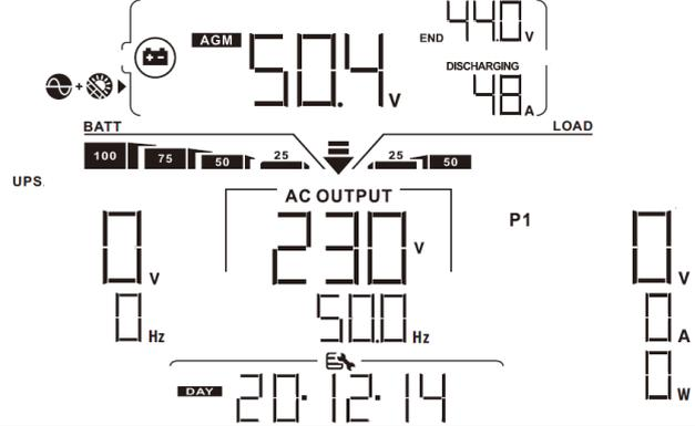
Load in VA=2.4kVA, Output frequency=50Hz
