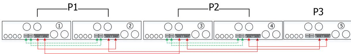
Two inverters in one phase and only one inverter for the remaining phases:
