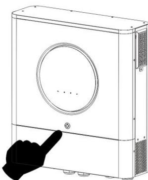
Step 4. Be sure to select battery type as "SOL" in LCD program 5.
