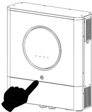
Step 4. Be sure to select battery type as "WEC" in LCD program 5.
