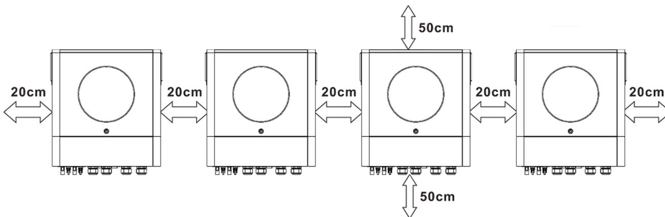
**NOTE:** For proper air circulation to dissipate heat, allow a clearance of approx. 20 cm to the side and approx. 50 cm above and below the unit. Be sure to install each unit in the same level.
