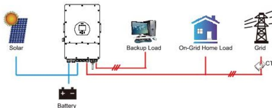
**Solar Sell:** "Solar sell" is for Zero export to load or Zero export to CT: when this item is active, the surplus energy can be sold back to grid. When it is active, PV Power source priority usage is as follows: load consumption and charge battery and feed into grid.
