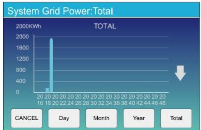
Solar power curve for daily, monthly, yearly and total can be roughly checked on the LCD, for more accuracy power generation, pls check on the monitoring system. Click the up and down arrow to check power curve of different period.
