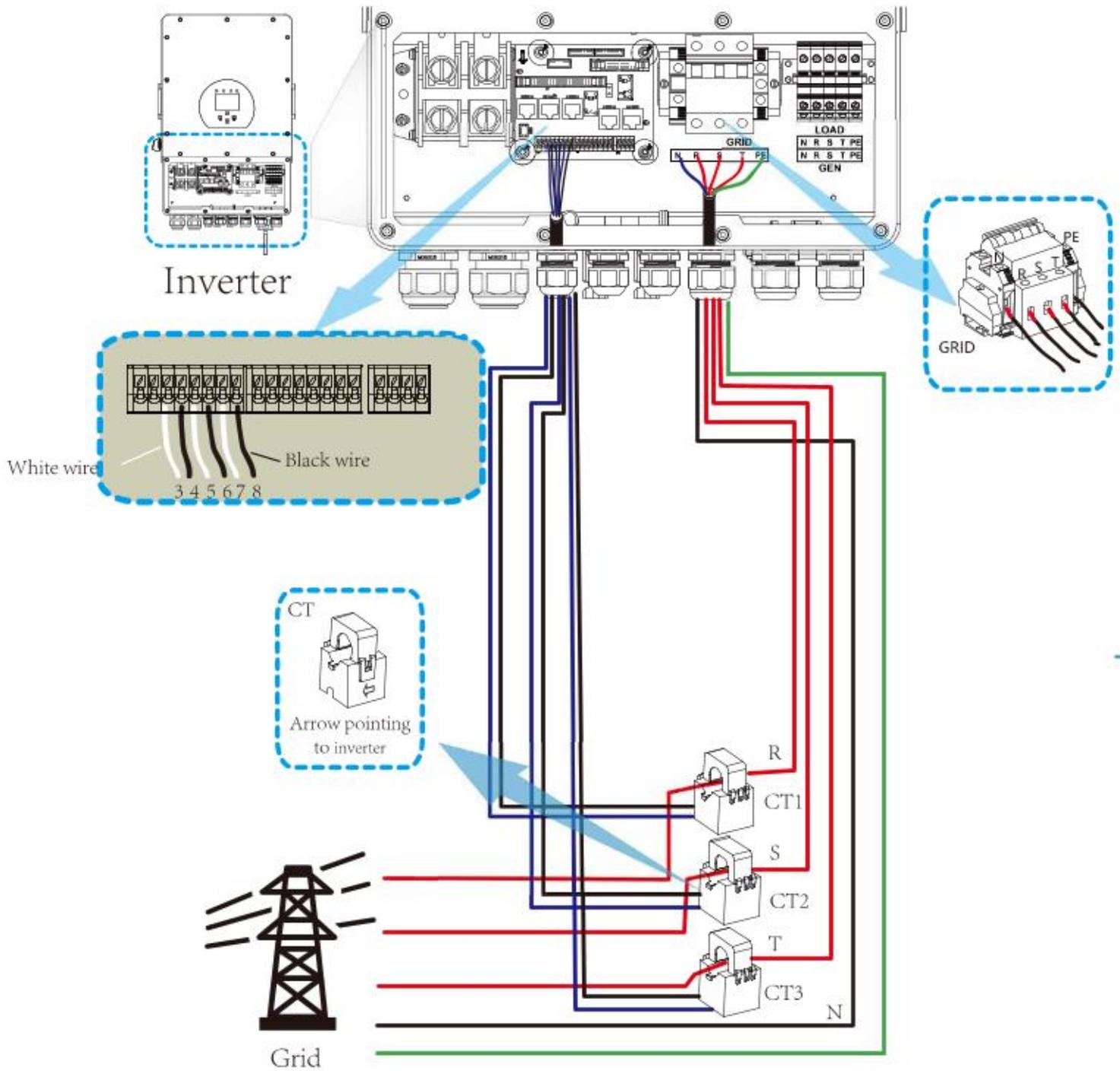
**\*Note:** when the reading of the load power on the LCD is not correct, please reverse the CT arrow.
